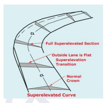
superelevations greater than 2% on all curves. We expect that most of the cross-grades greater than 2% can be easily corrected during the repaving process at a minimal cost relative to the current plan.
